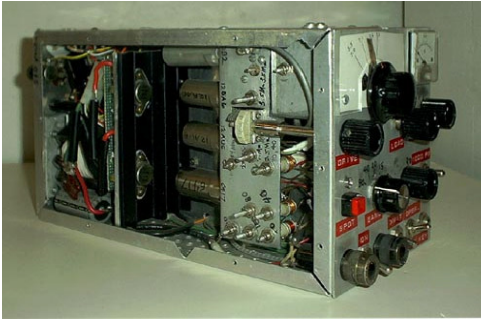
A 1967 homebrew all-band transmitter with a switching power supply running on 12 volts DC
