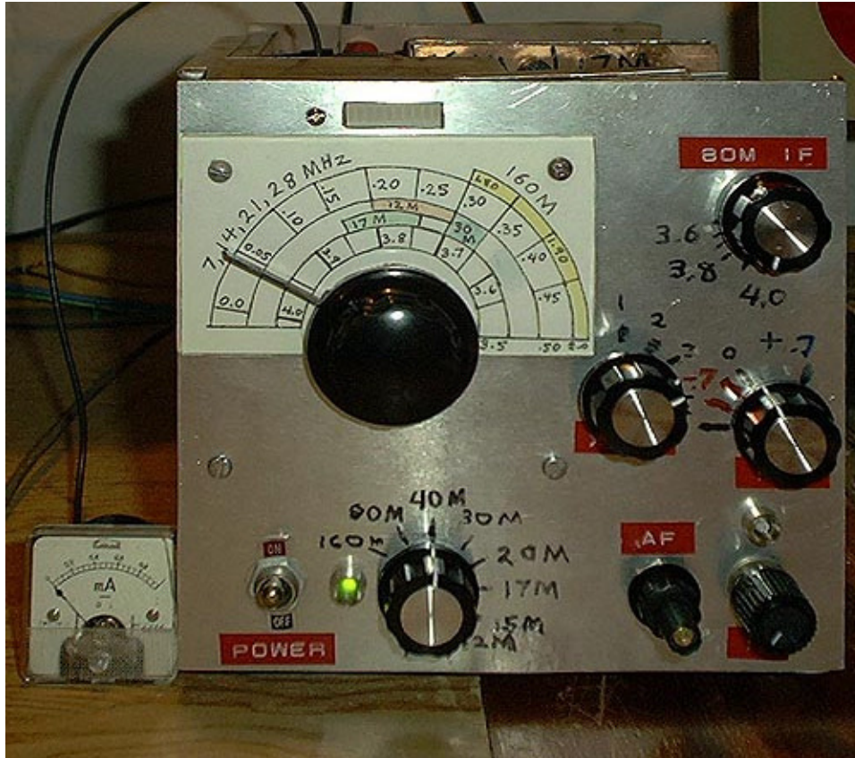
Homebuilt all-band dual conversion HF ham receiver.
