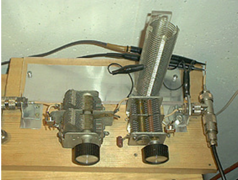
The T-Match monitored by oscilloscope and counter probes. The low pass filter is on the left. The antenna coaxial cable exits on the right.
