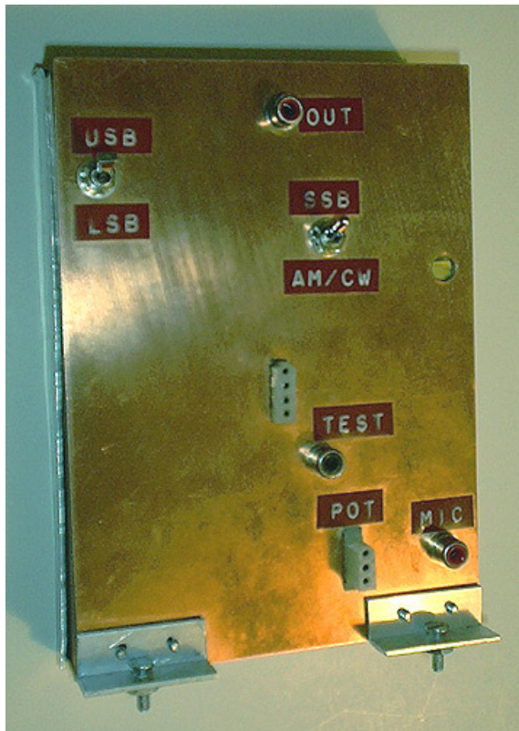
The 9 MHz SSB generator as seen from the control side
