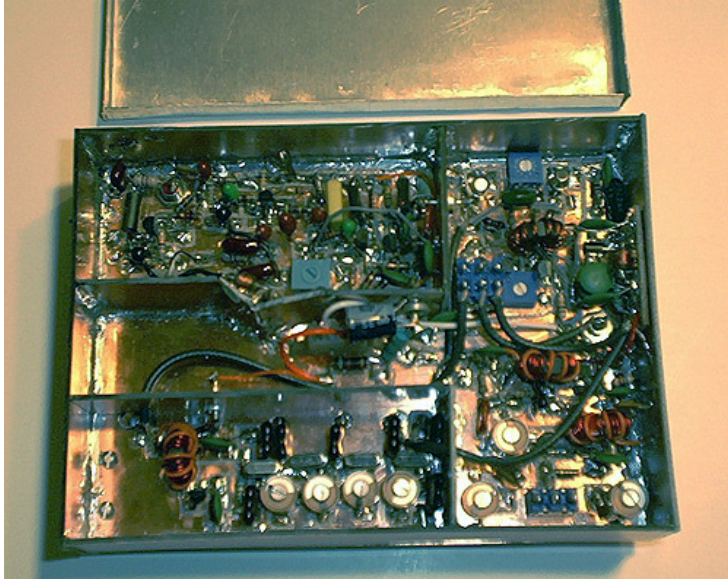
The completed 9MHz SSB generator. An aluminum lid fits over the top of the box.
